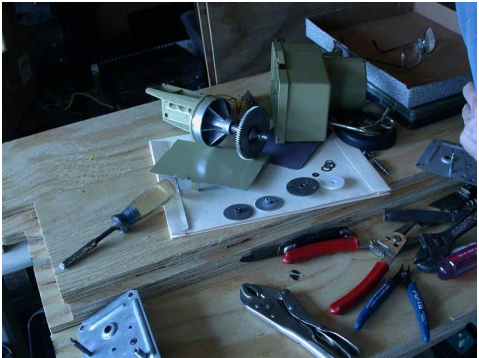
The gears de-greased and laid out on the workbench
